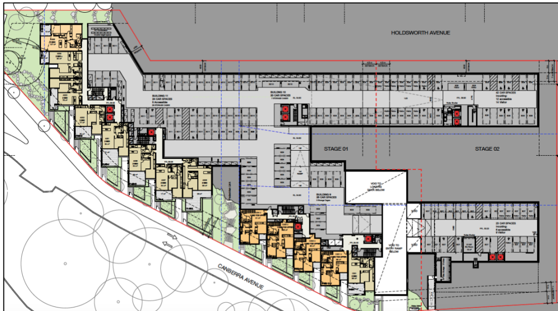
Figure 9. Typical Basement Design Source: Bates Smart
